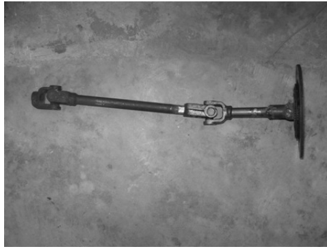
Fig 19: universal joint shaft welded to clutch plate.
